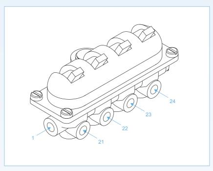
1 : air inlet21 : working port 122 : working port 223 : working port 324 : working port 4
